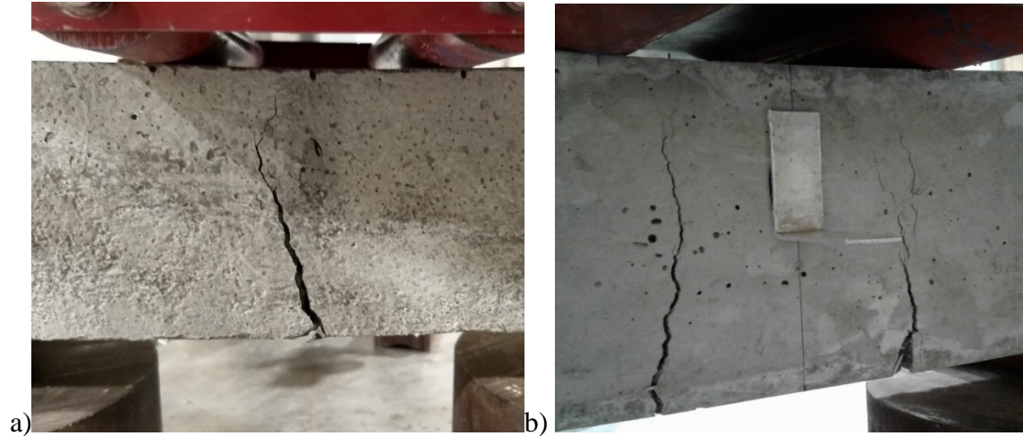
Figure 3.5 a) Single Crack Pattern Failure b) Double Crack Pattern Failure
